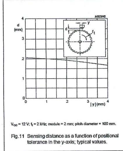
Fig.11 Sensing distance as a function of positional tolerance in the y-axis; typical values.
