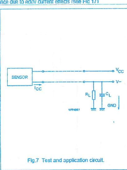
Fig.7 Test and application circuit.
