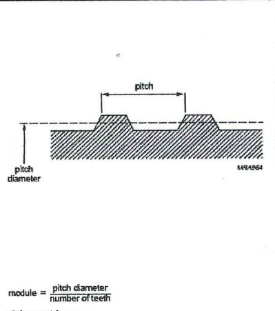
Fig.10 Gear wheel dimensions.
