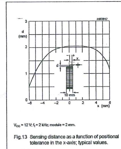
Fig.12 Sensing distance as a function of positional tolerance in the x-axis; typical values.
