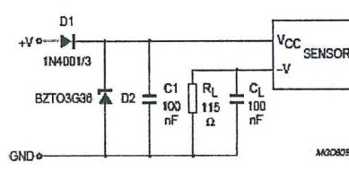
Fig.18 Test/application circuit for the KMI15/4.
