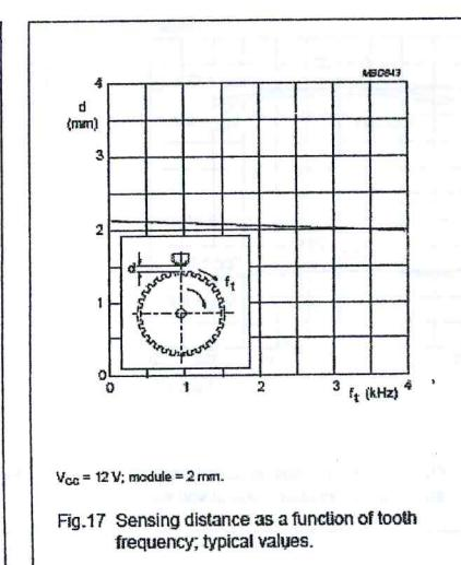
Fig.17 Sensing distance as a function of tooth frequency; typical values.
