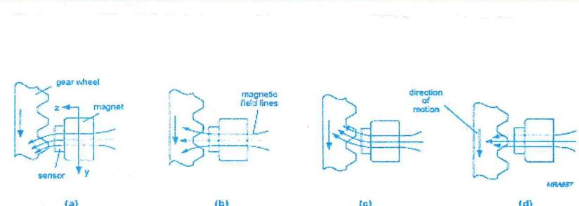
Fig.3 Functional principle.
