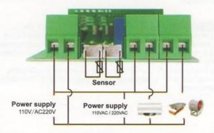
Note: There is no voltage output from the output terminal of the thermostat, So the device needs to be connected to a power supply
